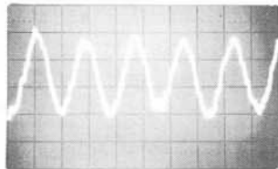
13 .05 V/cm, 2 \mu s/cm LOOP OPEN, OSC. COARSE SET FOR MAX 2nd HARMONIC
