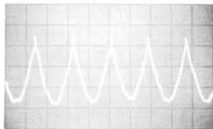
7 .5 V/cm, 2 ms/cm LOOP OPEN OSC. FINE at 300
